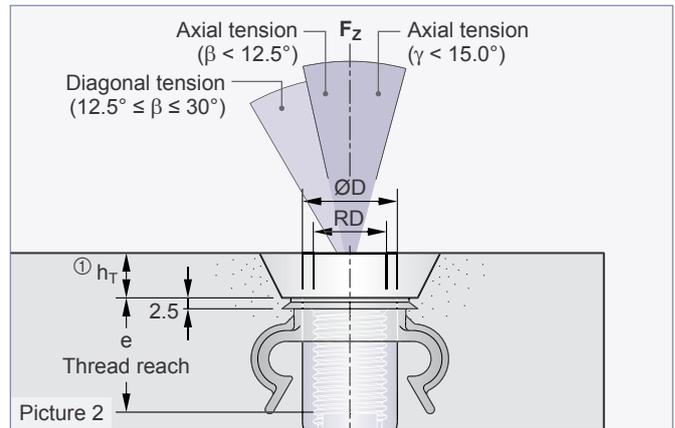
A threaded anchor with offset enables to balance an inclination of reinforced concrete sandwich panels during lifting and mounting.
